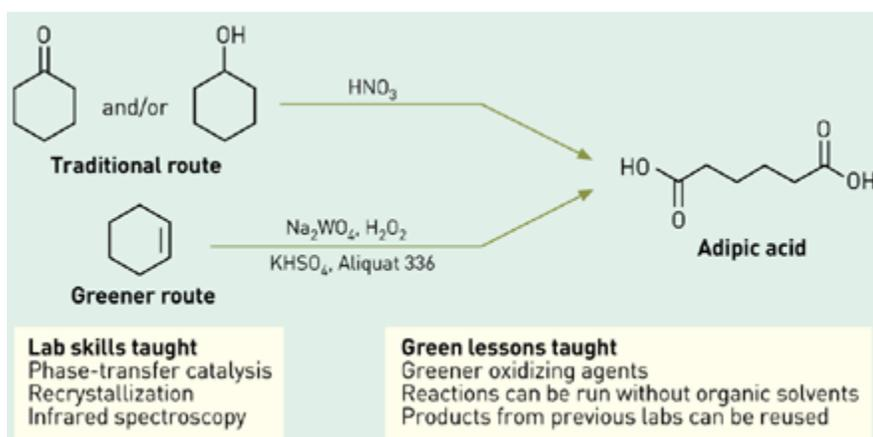
**MORE BENIGN** One of the green organic lab experiments developed at the University of Oregon is the synthesis of adipic acid, a feedstock used to make nylon. The experiment teaches the same lab skills as a traditional experiment while stressing the principles of green chemistry by avoiding production of nitrous oxide as a by-product and using only water as a solvent [*J. Chem. Ed.*, 77, 1627 (2000)].
