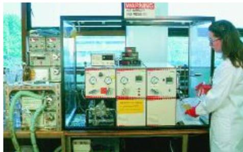
**SUPERCritical** Postgraduate student Eleni Venardou exchanges collection flasks at the supercritical water reactor used to make terephthalic acid at the University of Nottingham. The reactor uses a series of pumps to mix *p*-xylene, oxygen generated from hydrogen peroxide, water, and MnBr<sub>2</sub> catalyst, which pass through a high-pressure reactor. The reaction is the first selective oxidation to be carried out as a continuous process in supercritical water.
